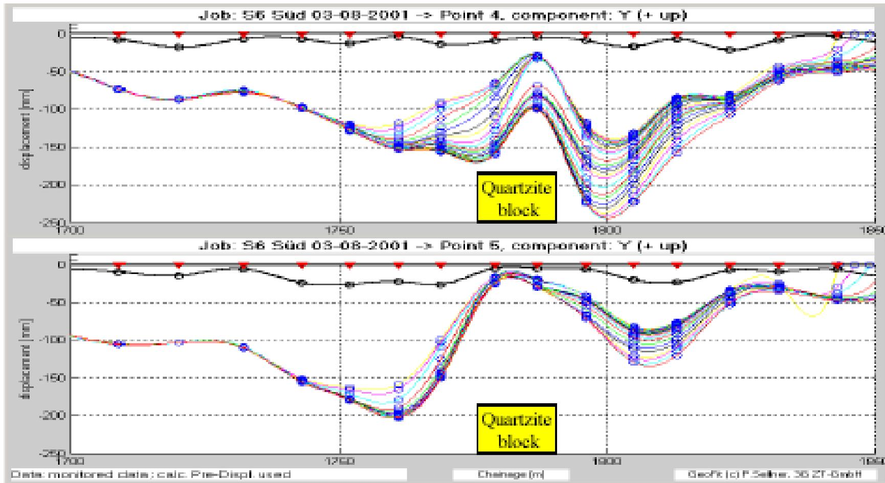
Figure 9. Deflection lines for points 4 and 5 showing the influence of the quartzite block located in the bench between stations 1771 and 1779 on the displacements.
