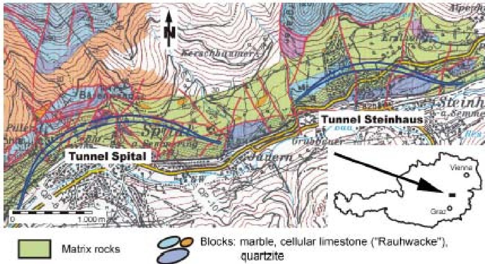
Figure 1. Site location and geology. The tunnel alignments are shown with dark blue, matrix rocks are undifferentiated phyllites, which surround blocks of marbles and rauhwaacke (dark and light blue) and quartzite (orange). Individual faults are identified with red lines.
