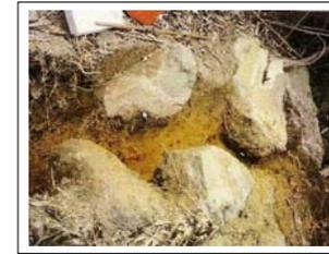
Medley & Sanz (2004) incorporated findings from Irfan & Tang (1993), who performed stability analyses of 10m high, 60 degree slopes in boulder colluvium. The model colluvium slopes contained uniformly sized and uniformly separated blocks, layered out-of-slope. Block proportions were varied between 10% and 55%. The strength properties of the matrix were generally  $c' = 5$  kPa and  $\phi' = 35$  degrees.
