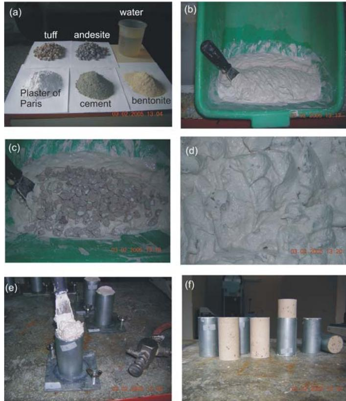
Fig. 2. Preparation stages of the artificial bimrock.
