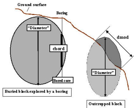
Fig. 2. Chords and  $d_{mod}$  compared to block “diameter” [4].
